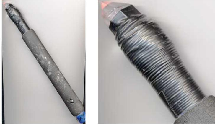
**Construction:** 15 inch long copper tube with crystal in top. Copper cap on bottom. Copper wire (18 gauge) wrapped around the top where the crystal mounts. This wire is then connected to one side of a krypton flashlight bulb mounted just under the crystal. The other side of the wire goes to the negative side of two AA nicad batteries located inside the copper tube. The positive of the nicad batteries goes to a small press switch mounted on the copper tube.
